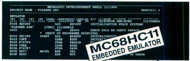
LE CONCEPT EMULATION ENTIERE EMBEDDED EMULATOR PERMET L'ECRITURE, LA MISE AU POINT, L'APPLICATION, LES CORRECTIONS SUR SITE ET L'EVOLUTION DU LOGICIEL DIRECTEMENT SUR RS232 D'UN PC SANS AUCUNE MANIPULATION DE CIRCUITS OU DE SONDAS, DIRECTEMENT PAR LA
