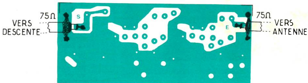
Figure 6 : Plan de câblage face raccordement.
