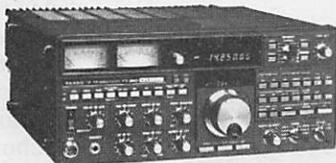
**YAESU - FT 290R.** Transceiver 144 MHz portable. Tous modes. 2 VFO. 2,5 W / 300 mW. 10 mémoires, accus et 13,8 V.
