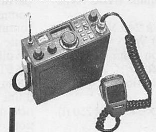
**YAESU - FT 209R.** Transceiver 144 MHz portable. FM. 3,5 W/300 mW (5 W / 500 mW en version RH).
