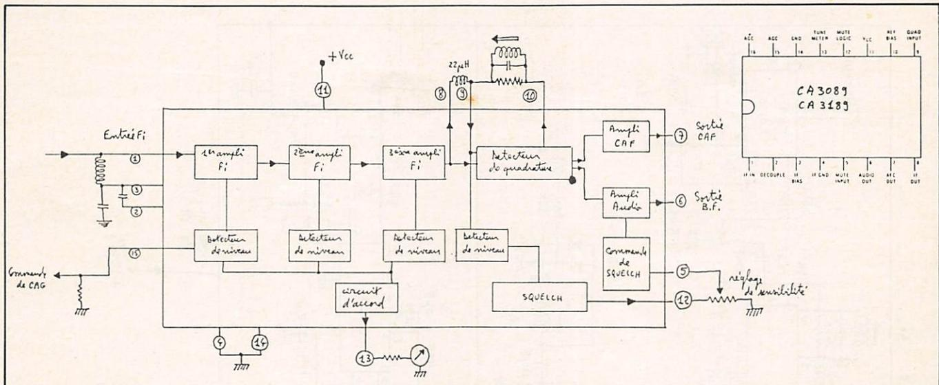
Figure 2 CA 3089 — DIAGRAMME DE FONCTIONNEMENT
